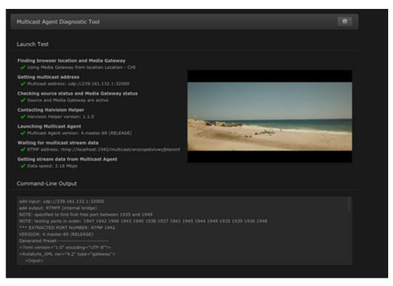
When the Multicast Agent Diagnostic Tool is opened, it performs a single test launch of the Multicast Agent and reports any failures due to bad HMP or user configuration, network issues, or other problems. It launches the Multicast Agent the same way that the normal HMP player does, but performs additional checks to help isolate problems with a multicast environment.
