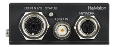
There is no power switch on the encoder. The power is automatically on when the unit is plugged in.
