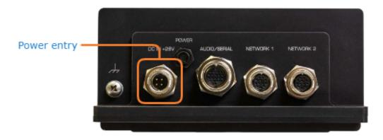
There is no power switch on the encoder. The power is automatically on when the unit is plugged in.
