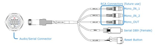
The Serial port is used to ingest KLV/CoT, as a management port or as pass-thru for camera control.
