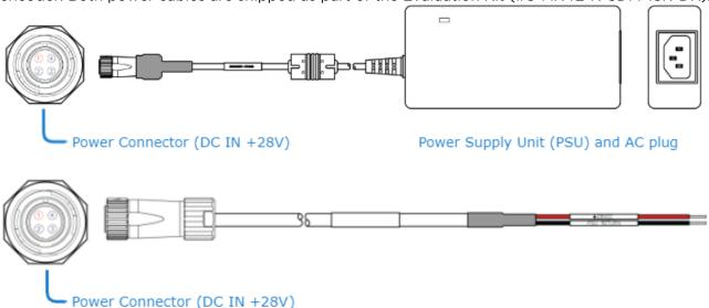
Make sure the connector is properly inserted and locked to avoid intermittent power problems.
