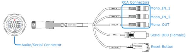
The Serial connector is used to ingest KLV/CoT, as a management port or as pass-thru for camera control.
