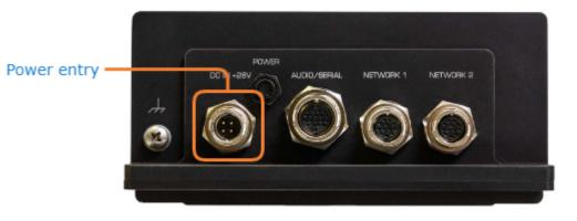
There is no power switch on the encoder. The power is automatically on when the unit is plugged in.
