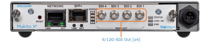
The HD-BNC connector(s) are used for SD-SDI (Serial Digital Interface), HD-SDI, 3G-SDI, 6G-SDI and 12G-SDI video output signals. All ports are 6/12G-SDI capable.
