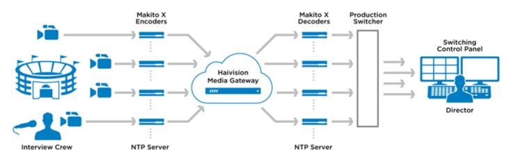
Two or more Makito X Series decoders can synchronize their output by using a frame buffer that holds a frame (or field if the signal is interlaced) momentarily until it falls into alignment with the other channels. This is accomplished by applying a fixed delay (referred to as *MultiSync Delay*) from the time the video is captured or encoded to the time it is ultimately displayed.
