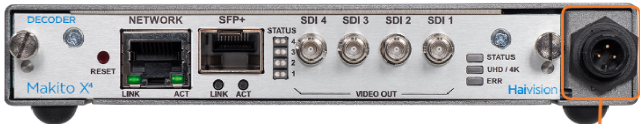
Connect Power Supply here (Power Input Jack)
