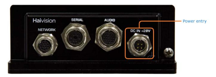
There is no power switch on the encoder. The power is automatically on when the unit is plugged in.
