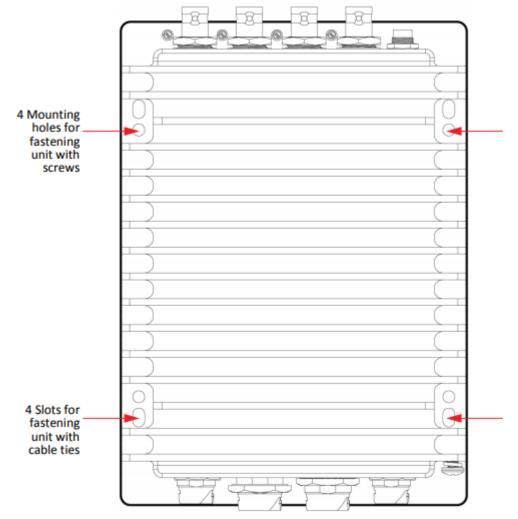
Or you can use two stainless steel, harsh-environment cable ties (up to 250 mils wide), which can be passed through slots in the chassis.
