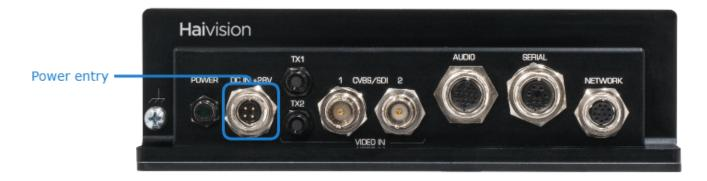
There is no power switch on the encoder. The power is automatically on when the unit is plugged in.
