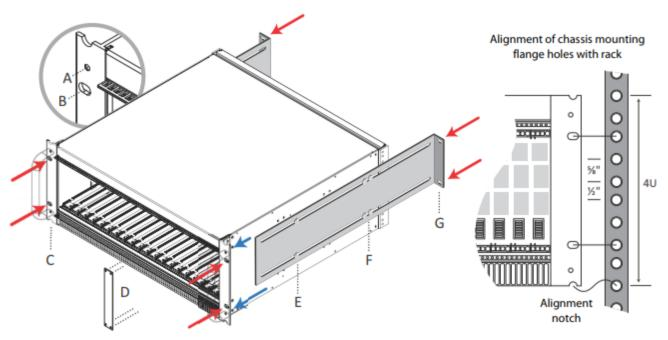
8. Loosely fasten the support brackets to the sides of the chassis with hex nut screws at (E) and (F). Slide them into place and secure them to the back of the rack (see red arrows in figure above; screws not provided).
