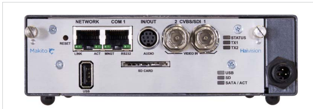
Figure 1-12 Dual SDI Appliance with Fixed (Internal mSATA SSD) Storage (#S-292E-SDI2-FS)
