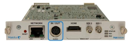
For the pinout, see Audio Connector Pinout.
