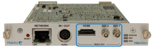
The audio is also embedded in the SDI and HDMI video. The SDI video supports up to 16 audio channels (8 pairs) and the HDMI supports 8 channels (4 pairs).
