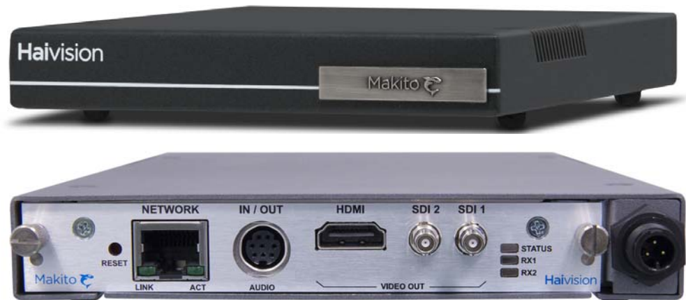
Figure 1-5 Front and Rear Views (Single Height Chassis, H.264, #S-292D-HD2)
