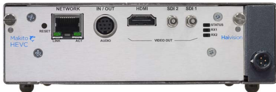
Figure 1-4 Rear View (Dual Height Chassis, H.264 and HEVC, #S-292D-HDI-HEVC)
