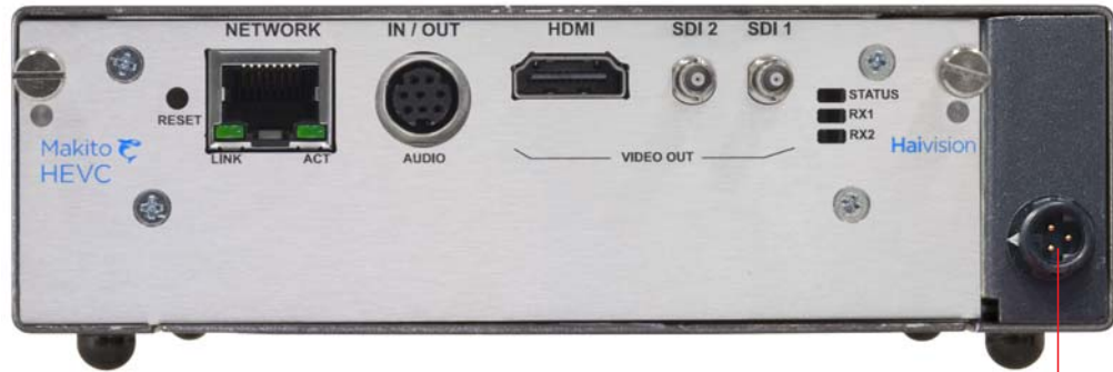
Figure 2-11 Rear Panel (Dual-Height Chassis, with Dual-Channel HEVC #S/B-292D-HD2-HEVC)
