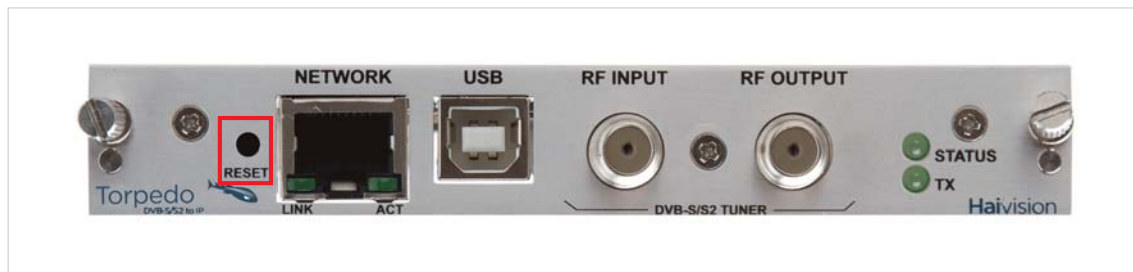
Figure 2-5 Reset micro switch (Sample view, Torpedo DVB-S/S2)
