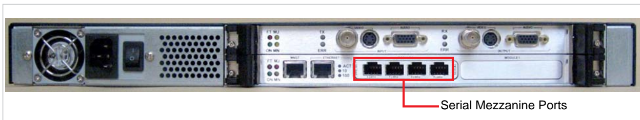
Figure 2-19 Sample hai1020 with Serial Data Mezzanine option
