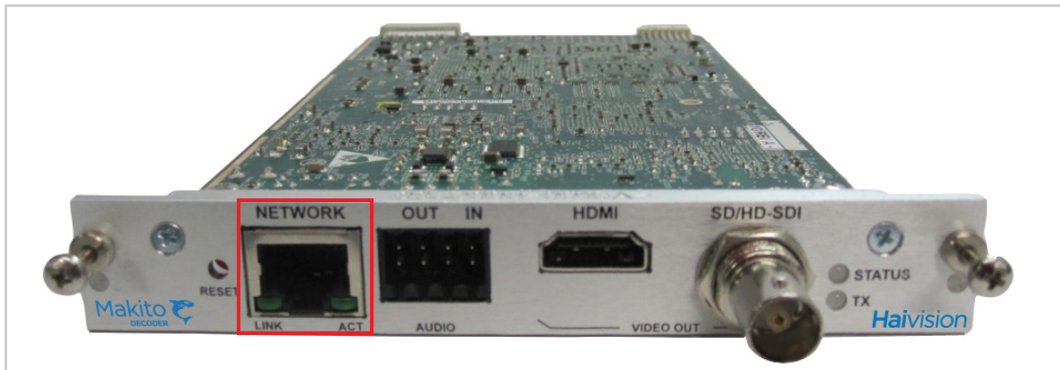
Figure 1-5 Ethernet Connection (Makito Decoder #B-290D)
