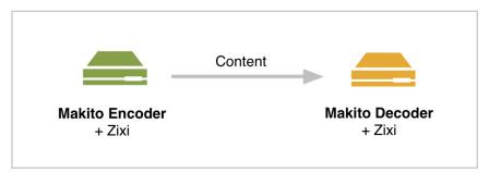
NOTE: The bitrate must be at least 1-8 Mbps for the stream bitrate for a single Zixi stream instance. You may optionally stream another stream type (such as TS/UDP) to a local server for recording.
