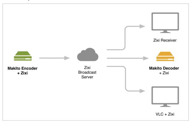
Point-to-Point-With Server: Makito Encoder to Makito Decoder direct unicast with broadcast server.
