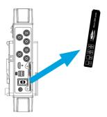
b) Insert SIM cards according to indications on cover.
