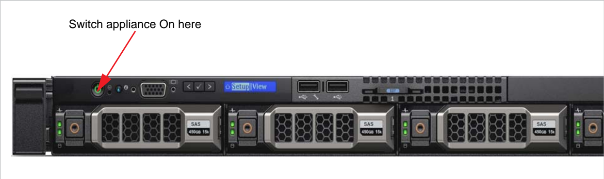
Figure 2-7 Sample Power Switch - Front panel (Portal Server)
