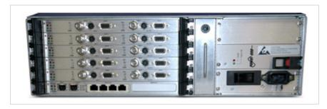
The Piranha captures metadata from the serial port interface and then incorporates the data information within the metadata elementary stream of the standard MPEG Transport Stream. The Serial Data Mezzanine supports four independent serial ports for KLV or CoT metadata capture. Note that only one serial input port can be used by each Encoder and that the same serial input port cannot be used by more than one Encoder.
